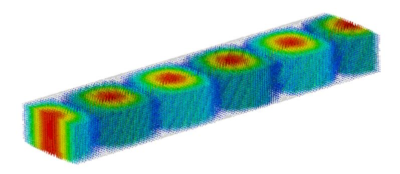
E-field phase animation inside a rectangular waveguide at 10 GHz.
