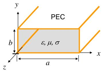
It is essentially an electromagnetic pipe with a rectangular cross-section.
