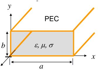
$$\left(\frac{\partial^2}{\partial x^2} + \frac{\partial^2}{\partial y^2}\right) h_z(x, y) = -k_c^2 h_z(x, y)$$
