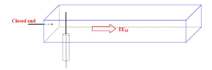
The inner conductor of the coaxial cable behaves like an antenna and it creates a maximum electric field in the middle of the crosssection.
